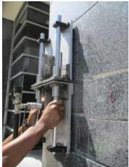
Fig. 5. ASTM C1823 Standard Test Method for Shear Bond Strength of Adhered Dimension Stone. Photos by Wiss Janney Elstner Associates, used with permission.
